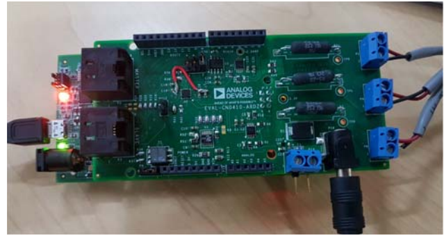
Figure 9. EVAL-CN0410-ARDZ Evaluation System
