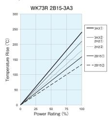
Regarding the temperature rise, the value of the temperature varies per conditions and board for use since the temperature is measured under our measuring conditions.
