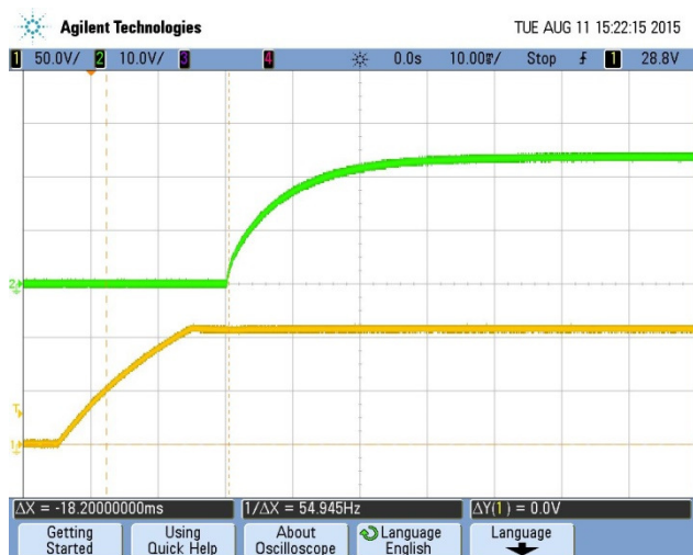
Figure 29: Turn-on transient at zero load current (10 mS/div, Top Trace: Vout, 10V/div; Bottom Trace: Vin, 50V/div)
