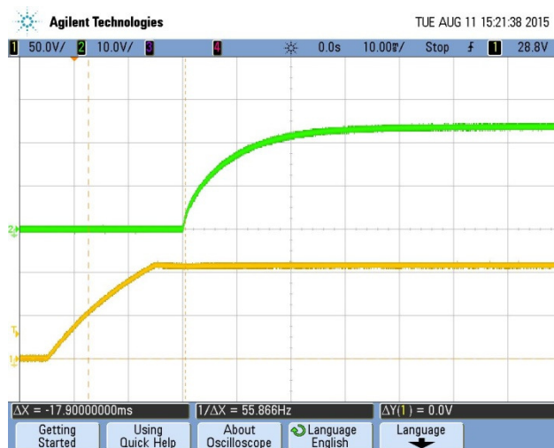
Figure 30: Turn-on transient at full load current (10 mS/div, Top Trace: Vout, 10V/div; Bottom Trace: Vin, 50V/div)
