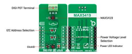
DIGI POT 13 Click communicates with the host MCU using the standard I2C 2-Wire interface, with a maximum clock frequency in Fast data transfer of up to 400KHz (400kbps). The I2C address can be selected via the ADDR SEL jumper with 0 selected by default. Over the I2C interface, all data can be stored in an internal 8-bit EEPROM.
