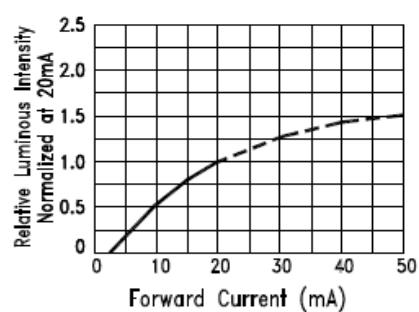
Fig.4 Relative Luminous Intensity
