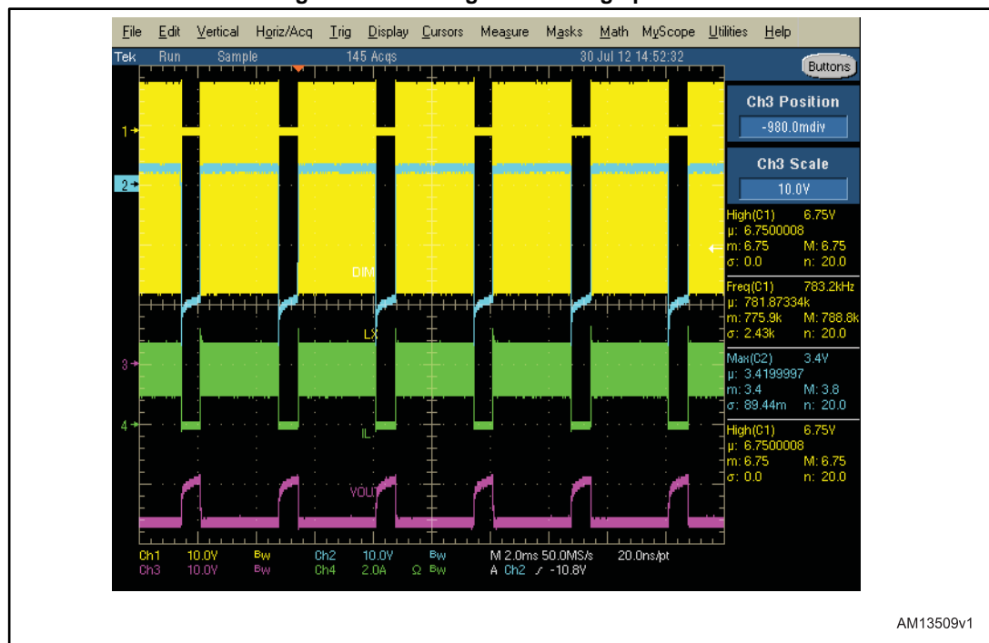
Figure 25: Inverting BB dimming operation
