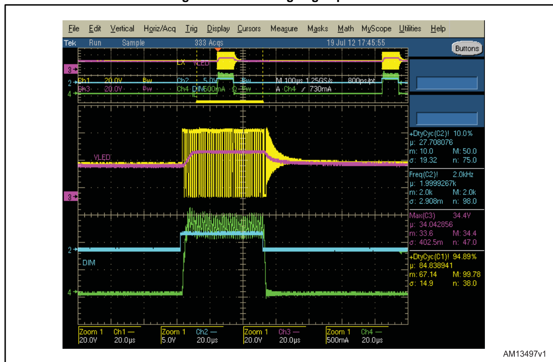
Figure 14: LED rising edge operation (zoom)
