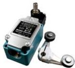
Enclosed Switches Series LS: Side Rotary with Yoke Style Lever; Steel Rollers; 1NC 1NO DPDT Snap Action, Maintained, Double Break; 20 mm [0.79 in] conduit; Compact/Non Plug-in
