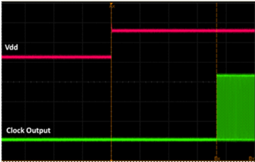
Figure 16. Startup Waveform vs. Vdd
