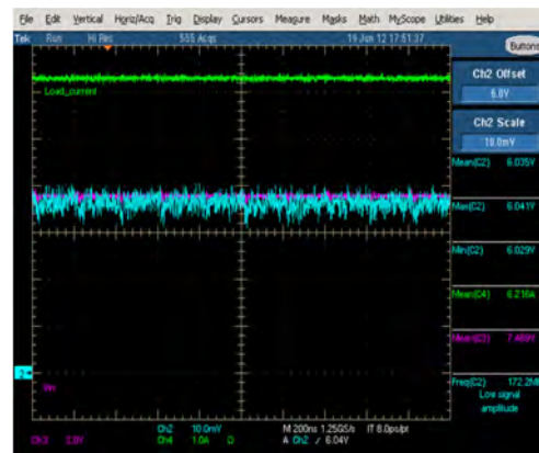
Figure 32. Ripple 8Vin Vo=6V, 6A 5MHz
