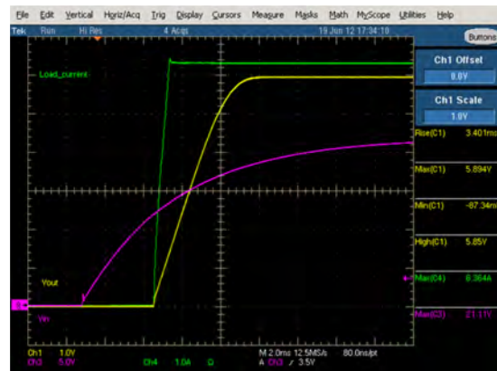
Figure 4. Start-up 22Vin Vo=5.8V, 6A, 5MHz
