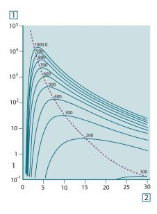
**Figure 33.6** Planckian curves plotted on semi-log scales from 100 K to 1000 K. The dotted line represents the locus of maximum radiant emittance at each temperature as described by Wien's displacement law. 1: Spectral radiant emittance (W/cm² ( $\mu$ m)); 2: Wavelength ( $\mu$ m).
