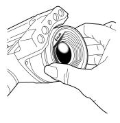
2. Rotate the lens 30° degrees counter-clockwise.
