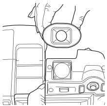
4. Carefully slide the eyecup into position.
