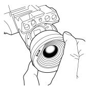
7. Carefully push the lens into position.
