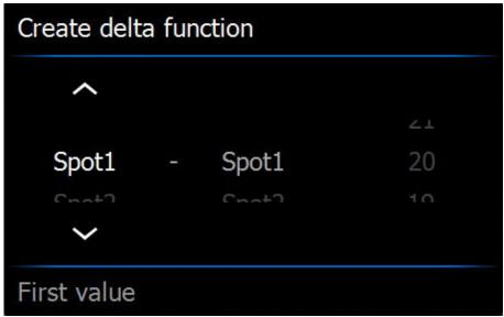
3. Push the joystick. The result of the difference calculation is now displayed on the screen.
