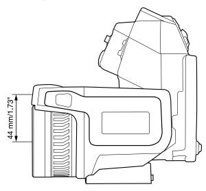
**Figure 8.1** This figure shows the difference in position between the laser pointer and the optical center of the infrared lens.
