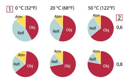
Figure 34.3 Relative magnitudes of radiation sources under varying measurement conditions (LW camera). 1: Object temperature; 2: Emittance; Obj: Object radiation; Refl: Reflected radiation; Atm: atmosphere radiation. Fixed parameters:  $\tau = 0.88$ ;  $T_{refl} = 20^{\circ}C$  (+68°F);  $T_{atm} = 20^{\circ}C$  (+68°F).
