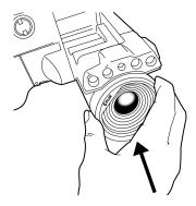
8. Rotate the lens 30° degrees clockwise.
