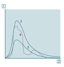
**Figure 33.8** Spectral radiant emittance of three types of radiators. 1: Spectral radiant emittance; 2: Wavelength; 3: Blackbody; 4: Selective radiator; 5: Graybody.
