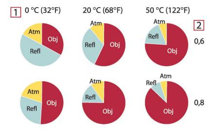
**Figure 34.2** Relative magnitudes of radiation sources under varying measurement conditions (SW camera). 1: Object temperature; 2: Emittance; Obj: Object radiation; Refl: Reflected radiation; Atm: atmosphere radiation. Fixed parameters:  $\tau = 0.88$ ;  $T_{refl} = 20^{\circ}C$  (+68°F);  $T_{atm} = 20^{\circ}C$  (+68°F).
