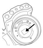
5. Note the index marks on the lens bayonet mount and on the lens.
