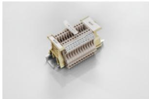
The SchT 5 S group tag carriers are clipped directly onto the TS 32 mounting rail (G-rail) or the TS 35 mounting rail (top-hat rail). It is therefore possible to label the terminal strip irrespective of the terminal and the type of terminal. SchT 5 and SchT 5 S are fitted with ESO 5, STR 5 protective strips.
