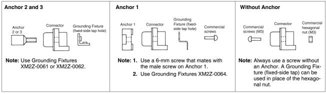
**Note: 1.** Anchor 2 and the following Grounding Fixtures are available: XM3B-22-11 and XM3B-22-112. Contact your OMRON representative for other anchor and grounding fixture specifications.
