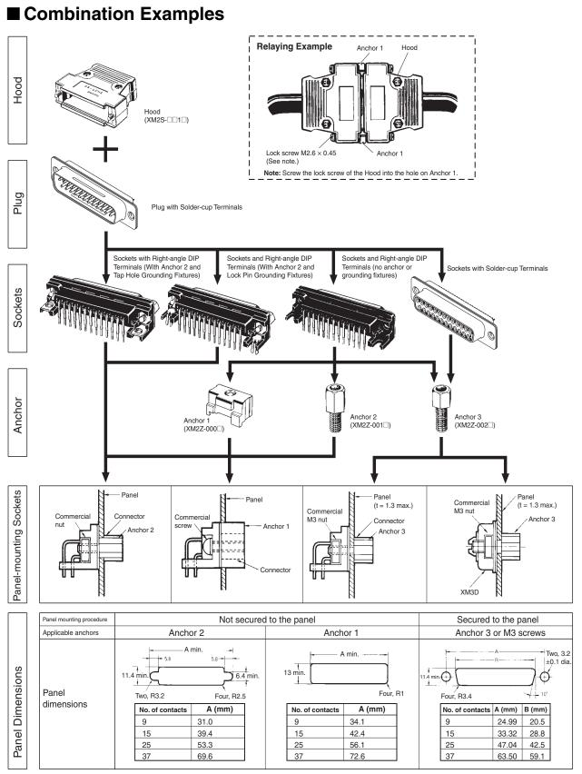
Note: 1. Two Anchors are required per Connector.
