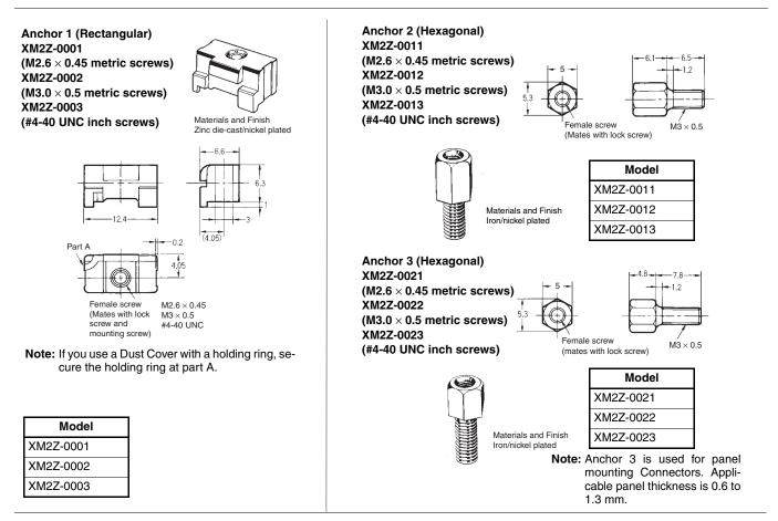
Note: 1. 2 anchors are necessary per connector.
