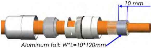
Step 4: Wrap foil over braided shielding
