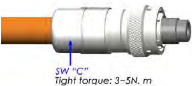
Step 9: Attach and tighten backshell as shown
