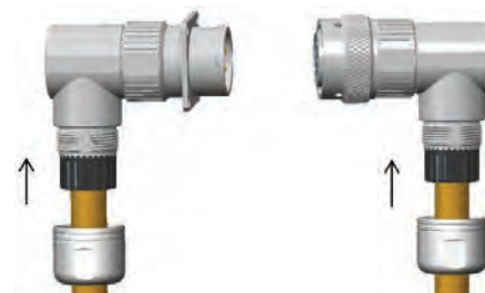
Step 12: Push cable grommet into backshell
