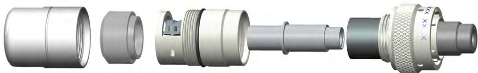
Step 1: Slide components onto cable
