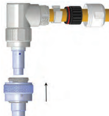
Step 12: Attach cable-nut to backshell and tighten as shown
