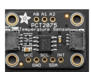
Primary Guide: Adafruit PCT2075 Temperature Sensor Is it hot in here or is it just you? Ask the PCT2075 temperature sensor!
