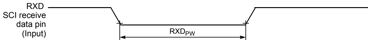
Figure 10-16 RXD Pulse Width
