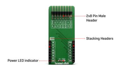
When there's a need to attach external equipment to the development system, the desired mikroBUS™ socket can be populated with Terminal click, allowing even more connections. This makes the stacking capacity almost unlimited. However, attention should be paid not to make the lines attached to the mikroBUS™ too long. In situations like this, the frequency of the communication might need to be stepped down a bit, in order to compensate for the longer mikroBUS<sup>™</sup> signal lines.
