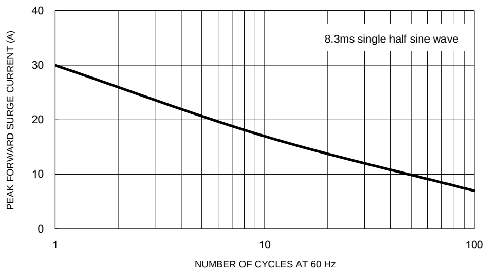
Fig.5 Maximum Non-Repetitive Forward Surge Current
