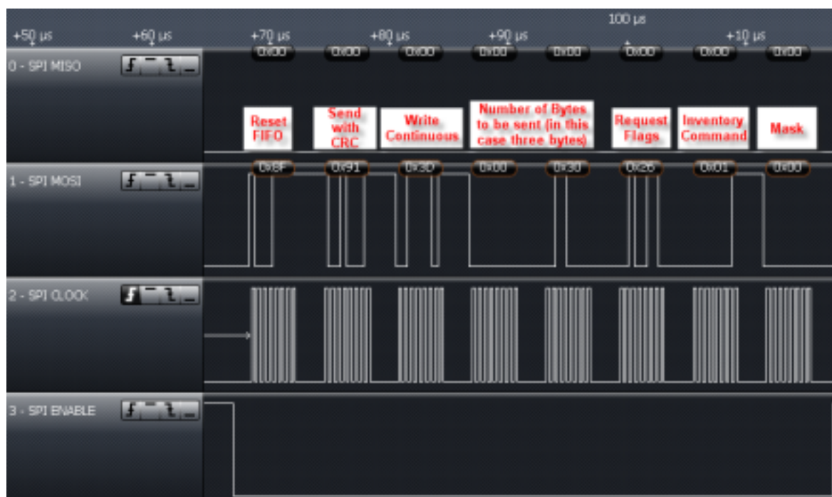
Figure 5-20. Inventory Command Sent From MCU to TRF7970A
