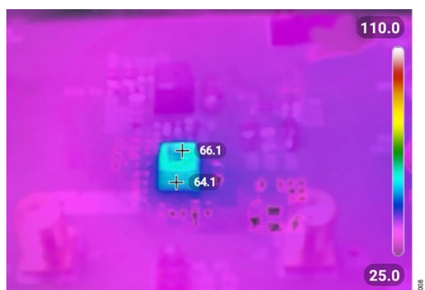
Figure 8. Thermal Image, 12V_{IN} , 1V_{OUT} , 12A Output, No Heat Sink, No Forced Airflow
