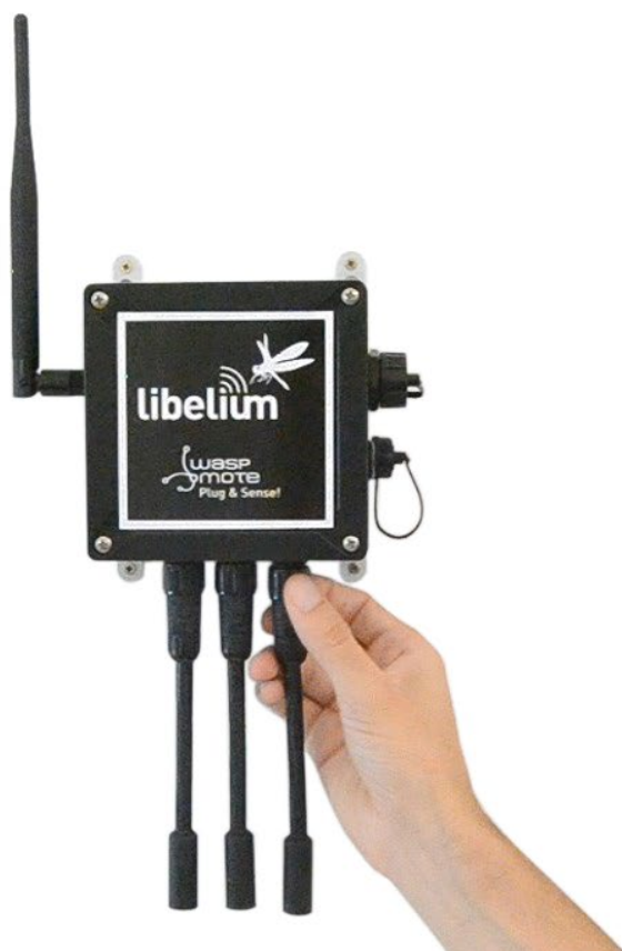
Figure: Connecting a sensor probe to Waspote Plug & Sense!
