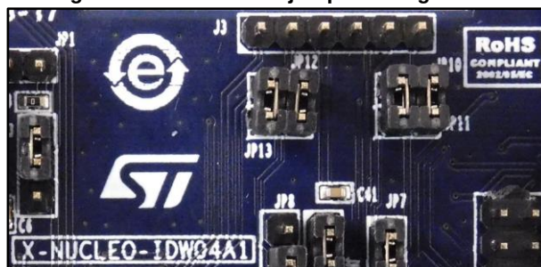
Figure 3: UART default jumper configuration
