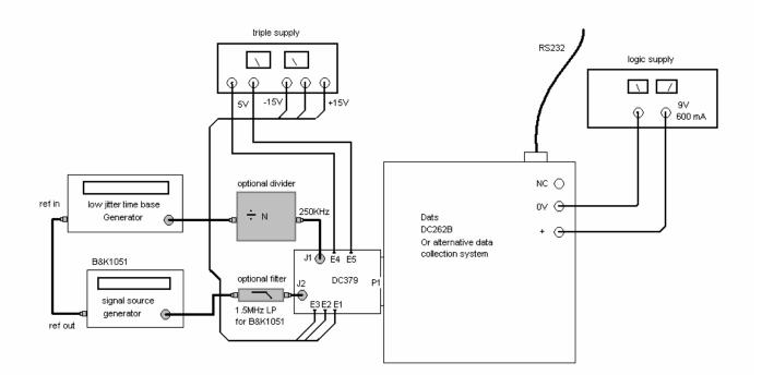
Figure 1. Proper Measurement Equipment Setup
