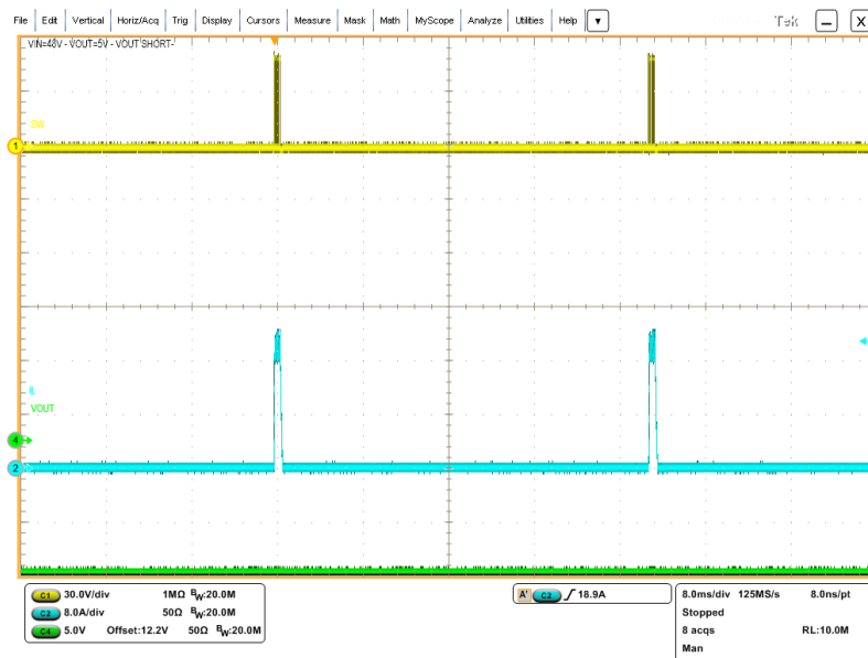
Figure 23. Hiccup in persistent short-circuit
