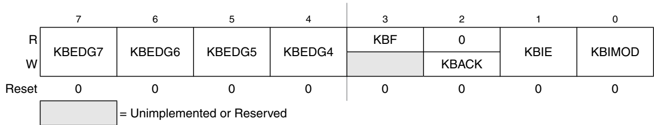
Figure 9-3. KBI x Status and Control Register (KBIXSC)
