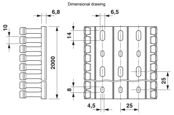
Base perforation according to DIN EN 50085
