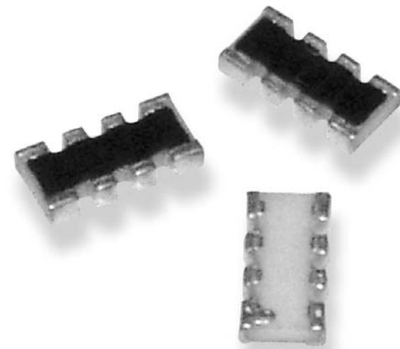
The MRS series is an entirely new chip network utilising nickel chrome sputtering on high purity alumina. This network has been designed for high volume applications and is offered with 4 isolated resistors on a single substrate (4 x 0603 resistors) at 0.1% with convex terminals. A wide value range and alternative TCRs (Temperature Coefficient of Resistance) make this a most versatile resistor solution.
