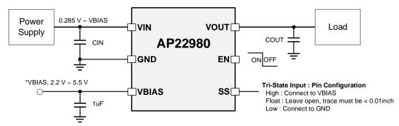
$<sup>^{\</sup>star}$  If  $V_{\text{IN}}$  is higher than 2.2V then VBIAS pin can be connected to VIN.
