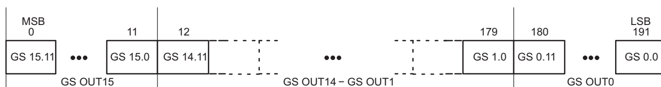
Figure 17. Grayscale Data Packet Format
