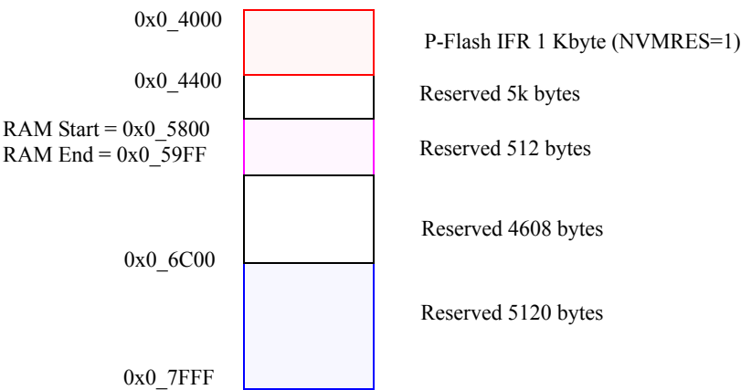
Figure 19-3. Memory Controller Resource Memory Map (NVMRES=1)
