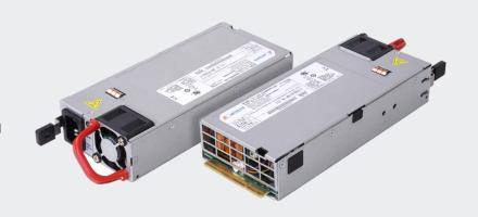
Advanced Energy's Artesyn DS495SPE is housed in 1U high rack-mounting enclosures measuring just 3.4 x 7.7 inches (86.3 x 196.5 mm). This form factor is significantly shorter than that of similarly rated earlier-generation power supplies — freeing up valuable system space — and is achieved by use of the latest power switching technology and high density component packaging techniques.
