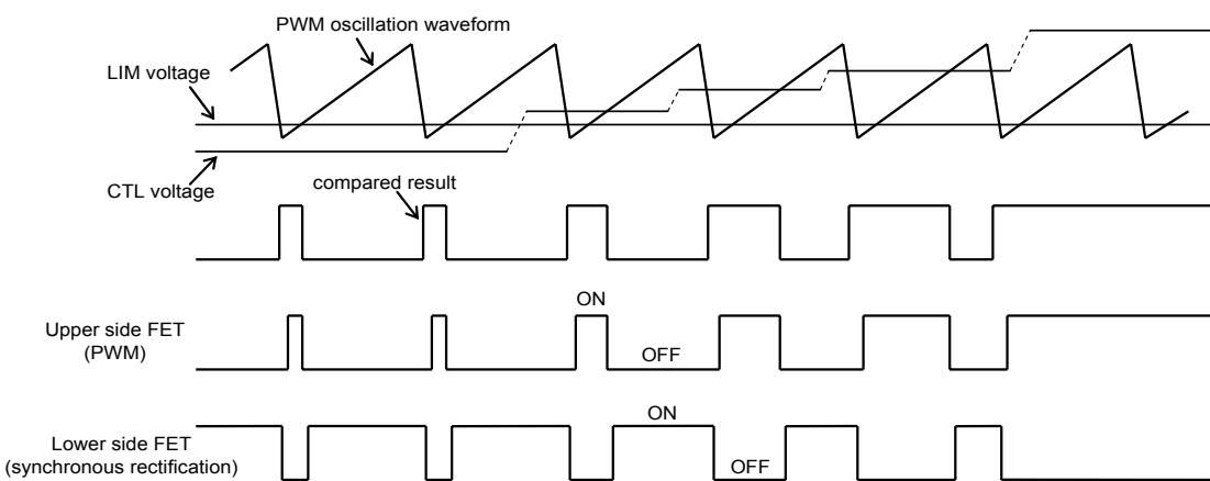
If a minus voltage is applied to the CTL pin, this pin current must be limited within 2mA by inserting the resistor of about 200Ω.
