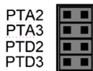
Figure 7-8: Jumper Settings for Input Signals to P&E's Embedded Multilink, P&E INPUT_EN (J11)
