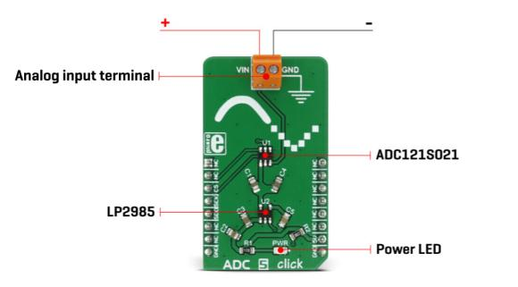
The ADC121S021 AD converter uses the SAR, or the successive approximation method for the conversion, which consists of comparing the input voltage with a series of internally generated voltage values. At each step in this process, the approximation is stored in a successive approximation register. The comparing steps are continued until the desired resolution is reached.
