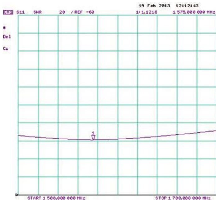
Antenna VSWR on Test Board
