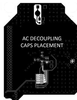
Figure 33. Example DS90UR241-Q1 EMC Layout
