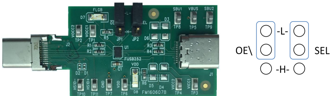
Figure 1 – Board Top View and DP/DM Select Pin Map
