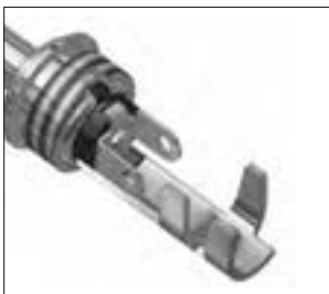
K-Series, Cable O.D 3mm to 5mm (0.118" to 0.196")
