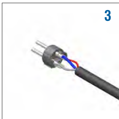
Solder the wires to the contacts.
