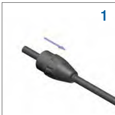
Slide the nut (Backshell) onto the cable
