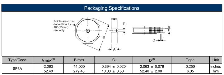
Dimension "E": This is a non-critical dimension that does not have a tolerance in the standard.
