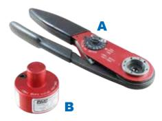
Heavy-duty M309 crimp tool for AWG size 8 to 18 wire. Adjustment wheel has 8 settings. Double action ratchet mechanism prevents improper crimps. Use with positioner, ordered separately.
