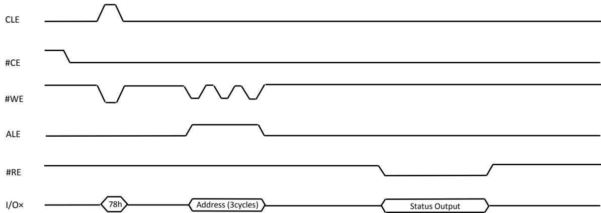
Figure 9-8 Read Status Enhanced (78h) Operation
