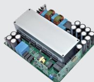
6.6kW High Power Density Bi-Directional EV On-Board Charger
