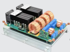
60kW INTERLEAVED BOOST CONVERTER CRD-60DD12N
