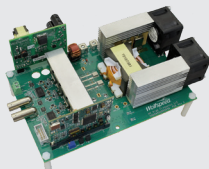
6.6kW High Frequency DC-DC Converter
