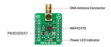
The MAX41470 has four power states: Shutdown, Sleep, Standby, and Receive-Active. Its Power-Down pin, labeled as PDN and routed to the RST pin of the mikroBUS™ socket, optimizes power consumption used for power ON/OFF purposes. When the device is enabled (the PDN pin set to a low logic state), the device operational states are controlled through the serial interface by the internal registers.
