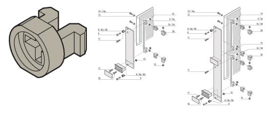
Sleeve guides the collar screw when fastening the front panel.
