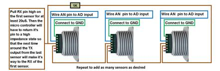
so on for all the sensor in the array. Once the last sensor has ranged, it will trigger the first sensor in the array to range again and will continue this loop indefinitely. Below is a diagram on how to set this up.
