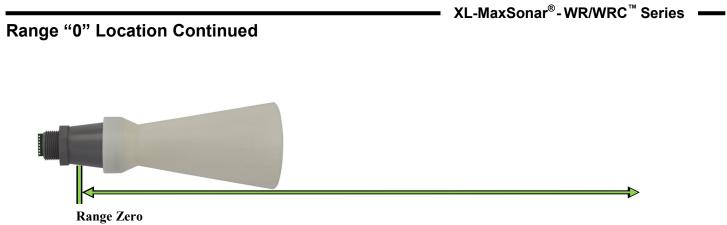
The range is measured from the front of the transducer to the target.
