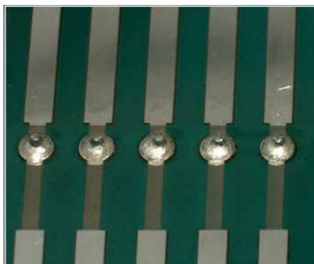
Solder joints on the bottom side of the PCB
