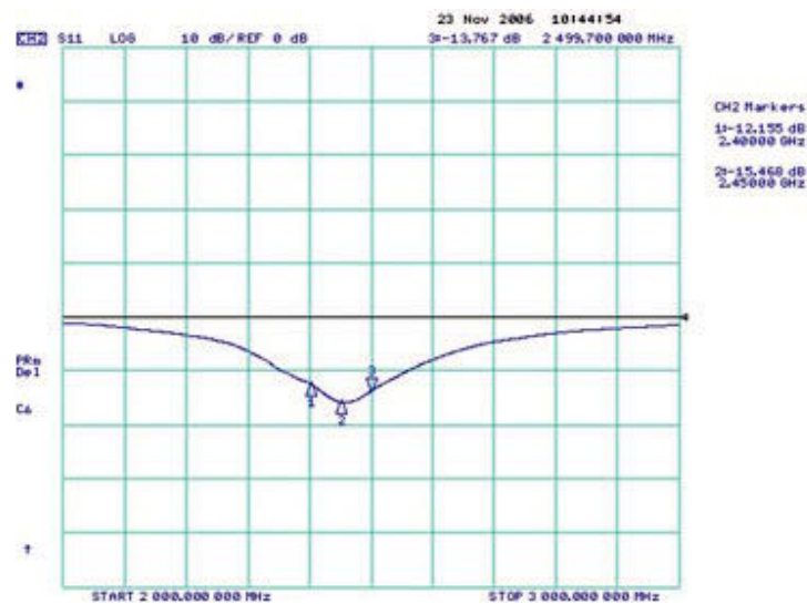
Antenna VSWR on Test Board
