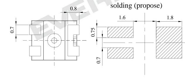
Note: Tolerances unless mentioned ±0.1mm. Unit = mm
