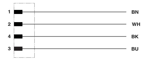
Contact assignment of the M12 plugs
