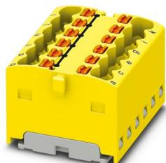
Distribution block, bridged internally, nom. voltage: 450 V, nominal current: 17.5 A, number of connections: 12, connection method: Push-in connection, cross section: 0.14 mm<sup>2</sup> - 2.5 mm<sup>2</sup>, mounting type: for snapping onto a DIN rail adapter, Direct mounting with flange, Free-hanging, color: yellow
