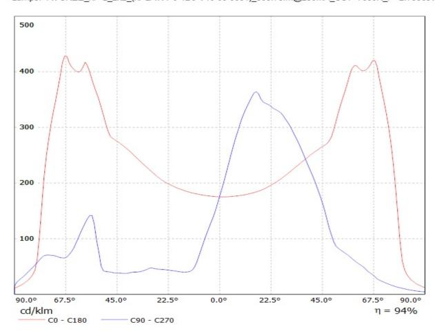
Luminaire: LEDiL Oy C13301\_STRADA-2x2-T3\_(XP-L) Lamps: 1 x CREE\_XP-L\_2x2\_(XPLAWT-0-1B0-V40-00-0001)\_514Im@250mA\_CCT=7600K\_P=2.79963W\_I=249.9mA
