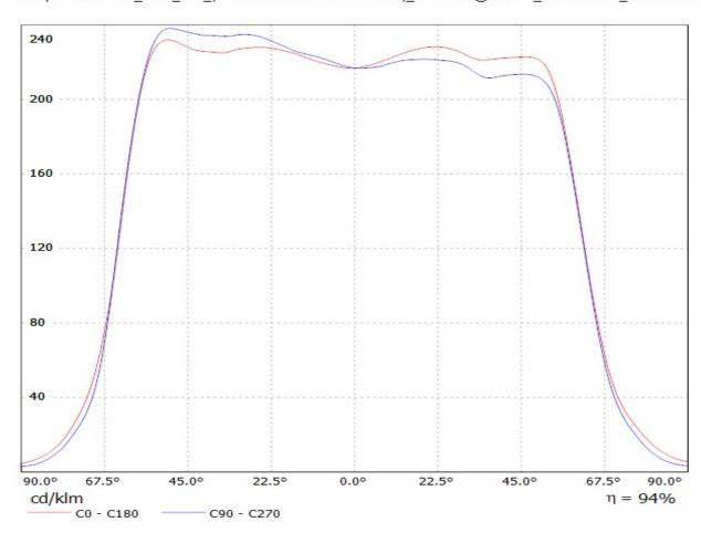
Luminaire: LEDiL Oy C13937\_STRADA-2x2-C-STP\_(XP-L) Lamps: 1 x CREE\_XP-L\_2x2\_(XPLAWT-0-1B0-V40-00-0001)\_504.373Im@250mA\_CCT=7600K\_P=2.79963W\_I=249.9mA
