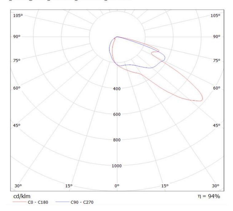
Luminaire: LEDiL Oy CS14143\_STRADA-IP-2X6-T3\_(XP-L) Eff.95.3% Lamps: 1 x CREE\_XP-L\_2x6\_(XPLAWT-0-7A3-U50-0H-0001) \_1270.8Im@250mA\_P=8.22317W\_I=249.8mA
