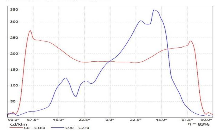
Luminaire: Ledil C15021\_STRADA-2X2-SCL\_(XP-L) Lamps: 1 x CREE\_XP-L\_2x2\_(XPLAWT-0-1B0-V40-00-0001) \_508.286lm@250mA\_CCT=7600K\_P=2.8173W\_I=0.25A
