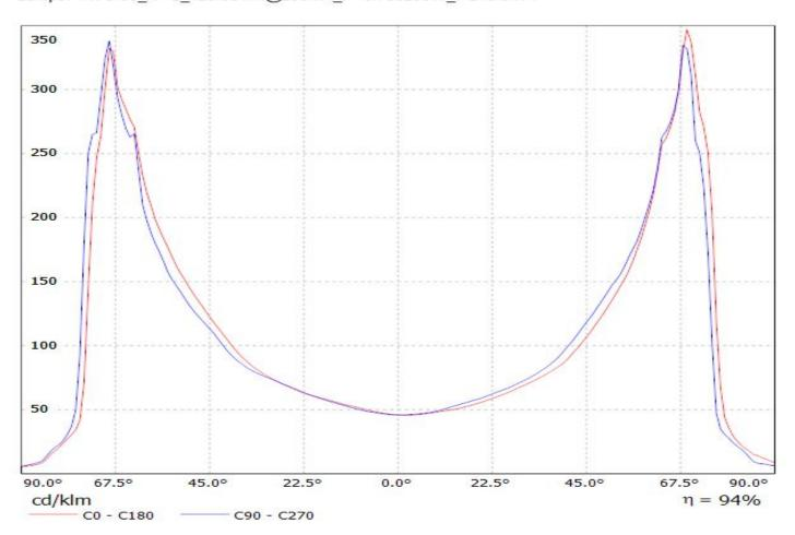
Luminaire: LEDiL Oy C12727\_STRADA-SQ-VSM\_(XP-L) Lamps: 1 x Cree\_XP-L\_130.23Im@250mA\_P=0.738255W\_I=249.9mA
