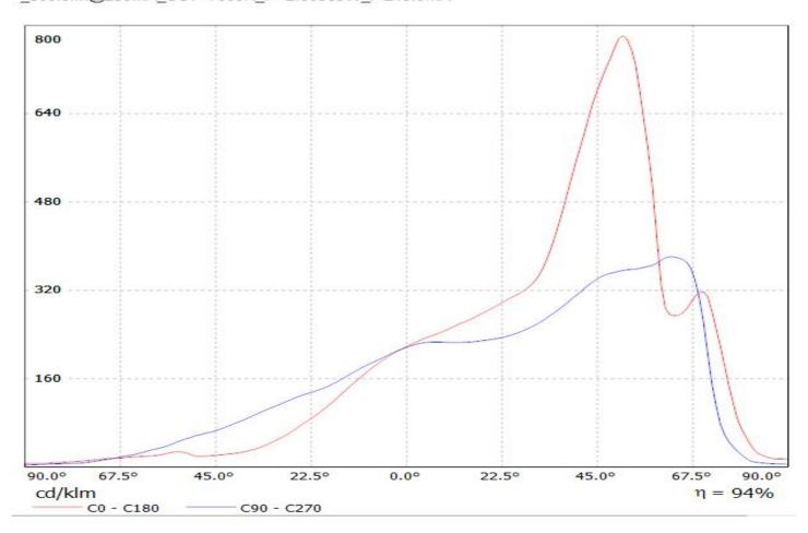
Luminaire: LEDiL Oy CS14143\_STRADA-IP-2X6-T3\_(XP-L) Eff.95.3% Lamps: 1 x CREE\_XP-L\_2x6\_(XPLAWT-0-7A3-U50-0H-0001) \_1270.8lm@250mA\_P=8.22317W\_I=249.8mA
