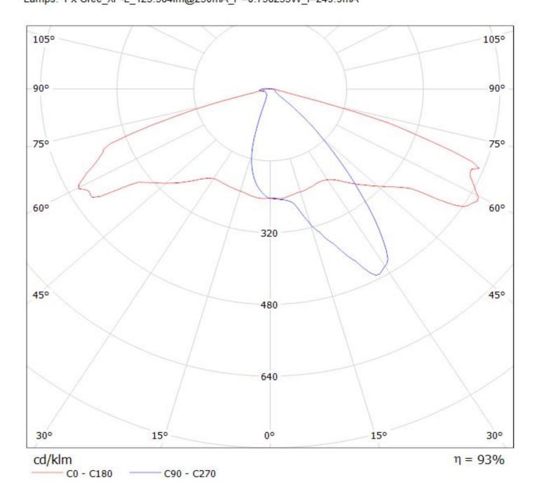
Luminaire: LEDiL Oy C13299\_STRADA-2X2-ME\_(XP-L) Lamps: 1 x CREE\_XP-L\_2x2\_(XPLAWT-0-1B0-V40-00-0001)\_518.95Im@250mA\_CCT=7600K\_P=2.79963W\_I=249.9mA
