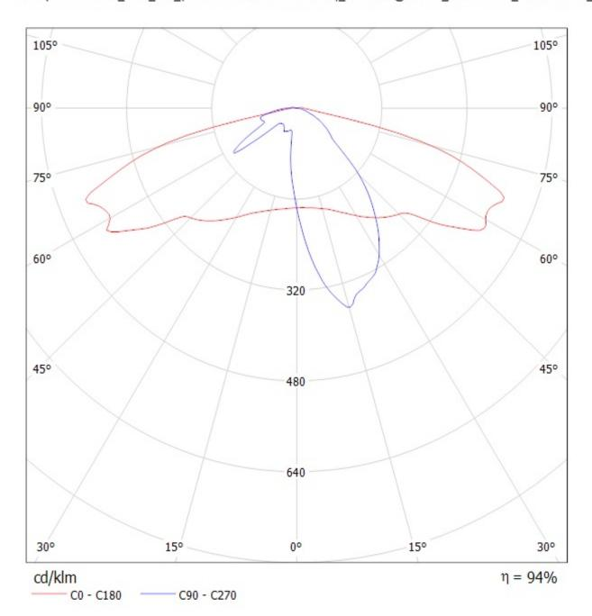
Luminaire: LEDiL Oy C13301\_STRADA-2x2-T3\_(XP-L) Lamps: 1 x CREE\_XP-L\_2x2\_(XPLAWT-0-1B0-V40-00-0001)\_514Im@250mA\_CCT=7600K\_P=2.79963W\_I=249.9mA
