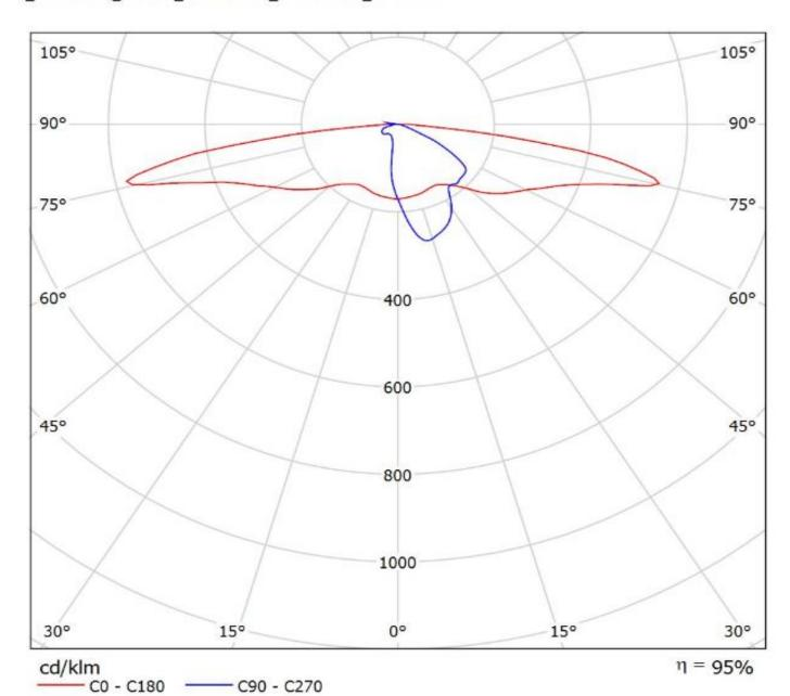
Luminaire: Ledil C15021\_STRADA-2X2-SCL\_(XP-L)\_glass Lamps: 1 x CREE\_XP-L\_2x2\_(XPLAWT-0-1B0-V40-00-0001) \_508.286lm@250mA\_CCT=7600K\_P=2.8173W\_l=0.25A
