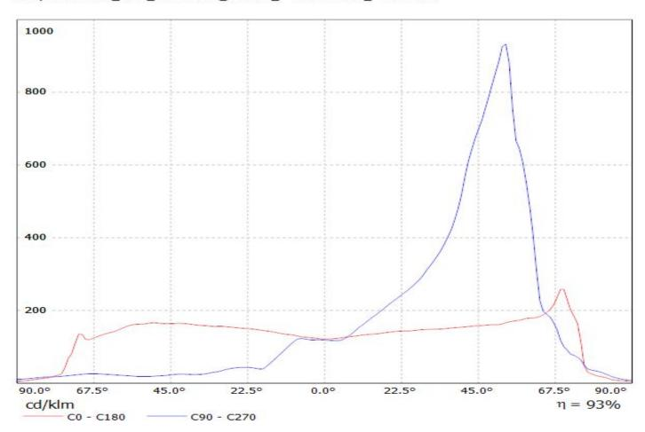
Luminaire: LEDiL Oy C13805\_STRADA-2x2-T4\_(XP-L) Lamps: 1 x CREE\_XP-L\_2x2\_(XPLAWT-0-1B0-V40-00-0001)\_515Im@250mA\_CCT=7600K\_P=2.79963W\_I=249.9mA
