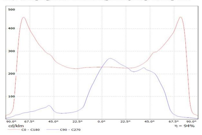
Luminaire: Ledil Oy CS15689\_STRADA-IP-2X6-FW\_(XP-L)\_SIMULATED Lamps: 1 x Cree XP-L
