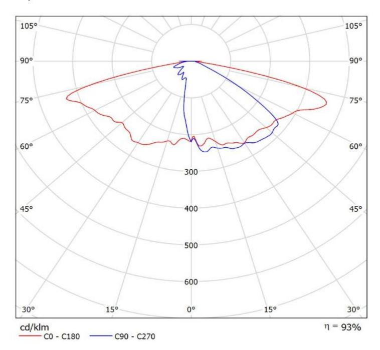
Luminaire: LEDiL Oy CA14843\_STRADA-B2\_(XP-L)\_Cav2 Lamps: 1 x Cree\_(XP-L)\_123.939Im@250mA\_P=0.736105W\_I=0.2499A
