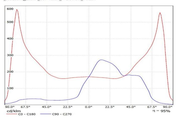
Luminaire: Ledil C15021\_STRADA-2X2-SCL\_(XP-L)\_glass Lamps: 1 x CREE\_XP-L\_2x2\_(XPLAWT-0-1B0-V40-00-0001) \_508.286lm@250mA\_CCT=7600K\_P=2.8173W\_I=0.25A
