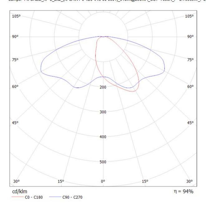
Luminaire: LEDiL Oy C12362\_STRADA-2X2-DWC\_(XP-L) Eff.94.2% Lamps: 1 x CREE\_XP-L\_2x2\_(XPLAWT-0-1B0-V40-00-0001)\_504.373lm@250mA\_CCT=7600K\_P=2.79963W\_I=249.9mA
