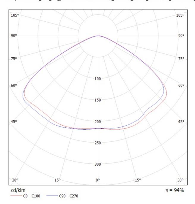
Luminaire: LEDiL Oy C13937\_STRADA-2x2-C-STP\_(XP-L) Lamps: 1 x CREE\_XP-L\_2x2\_(XPLAWT-0-1B0-V40-00-0001)\_504.373Im@250mA\_CCT=7600K\_P=2.79963W\_I=249.9mA
