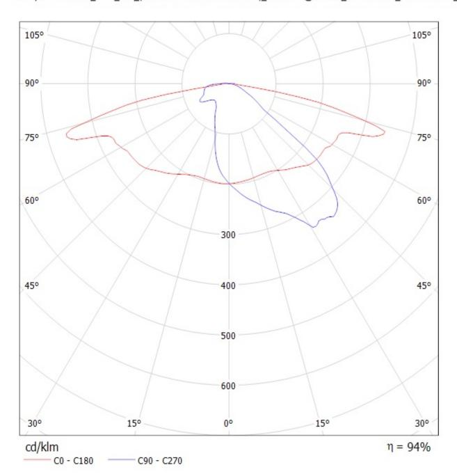
Luminaire: LEDiL Oy C13300\_STRADA-2x2-T2\_(XP-L) Lamps: 1 x CREE\_XP-L\_2x2\_(XPLAWT-0-1B0-V40-00-0001)\_508.75Im@250mA\_CCT=7600K\_P=2.79963W\_I=249.9mA
