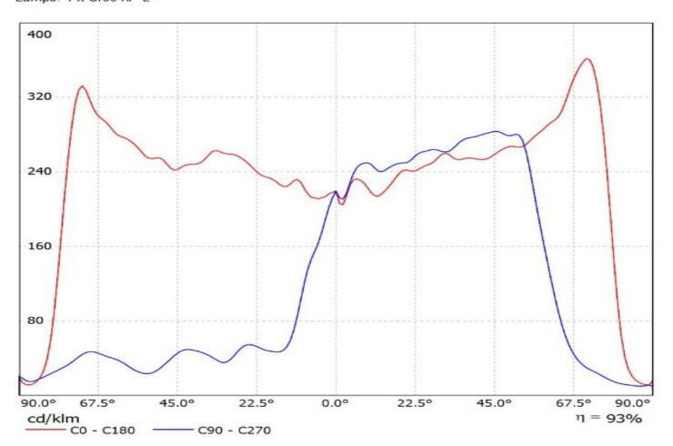
Luminaire: LEDiL Oy CA14843\_STRADA-B2\_(XP-L)\_Cav2 Lamps: 1 x Cree\_(XP-L)\_123.939Im@250mA\_P=0.736105W\_I=0.2499A
