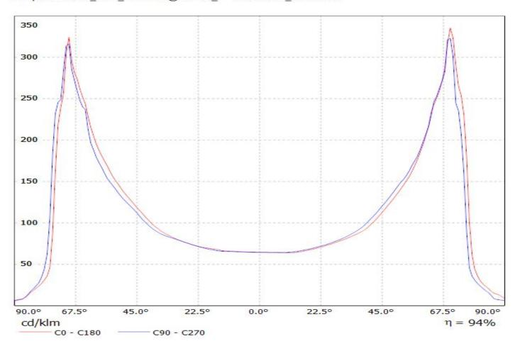
Luminaire: Ledil Oy C14165\_STRADA-2X2-ME-WIDE2\_(XP-L)\_SIMULATED Lamps: 1 x Cree XP-L
