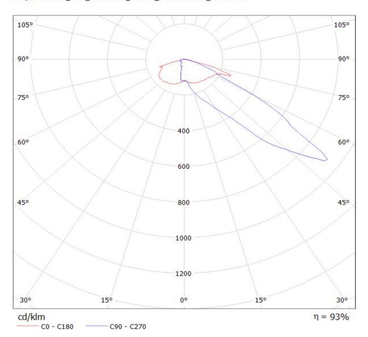
Luminaire: LEDiL Oy C13805\_STRADA-2x2-T4\_(XP-L) Lamps: 1 x CREE\_XP-L\_2x2\_(XPLAWT-0-1B0-V40-00-0001)\_515Im@250mA\_CCT=7600K\_P=2.79963W\_I=249.9mA
